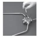
The Frame cannot be further disassembled into individual parts. Before you insert the Frame with the fixing arm into the coupling clamp of the table post, you should load the  $CO_2$ -Cylinder. Therefor you insert the Cylinder into the round opening at the top end of the pressure housing, set the locking cap onto the Cylinder and screw by hand. After tightening the locking cap, both of retractor arms and fixing arm are fixed.
